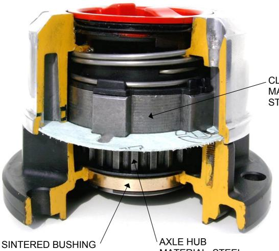
**CLUTCH RING** MATERIAL: MACHINED STEEL BAR
